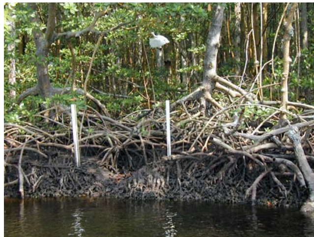
Figure 2. Permanent end posts either side of a routinely sampled intertidal rivulet: posts accommodate block net for capturing fish and crustaceans leaving the mangrove forest on an ebb tide.
