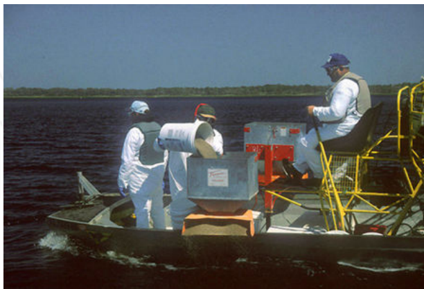
Figure 17. Application of granular herbicide using a boat-mounted spreader. Photo courtesy UF/IFAS Center for Aquatic and Invasive Plants.
